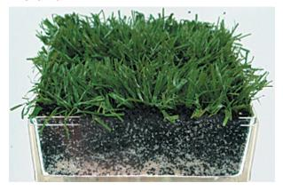
FieldTurf is a 100% recyclable artificial grass system made of polyethylene fibers which are durable yet soft to the touch. The infill is made from graded silica sand and cryogenically frozen and crumbled recycled rubber to provide a non-compactable, resilient, natural-feeling "synthetic earth" to withstand the most demanding environments.
