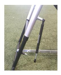
Step #8. Install each of the gas shocks. Note the cylinder end of the shock attaches to the silver tube and the rod end attaches to the black frame. The socket ends of the gas shocks simply snap over the ball studs.
