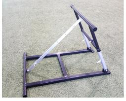
Step #6. Using the short 5/16" bolts, washers, and nuts, install the height strap assembly to each of the frame pieces. Once the nut is tightened loosen it 1/4 turn to allow movement when adjusting the height of the Seesaw.
