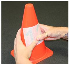
4. Starting at the edge of the pre-mask, slowly peel away the pre-mask at a low angle so you don't lift up the number. Discard the pre-mask sheet.
